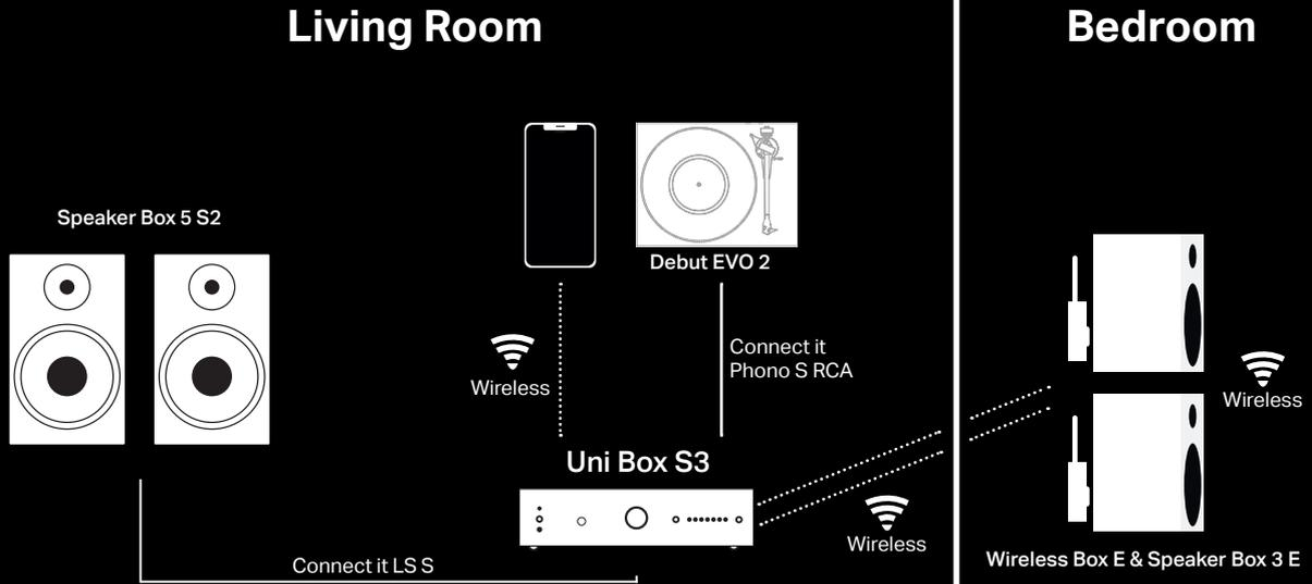
Uni Box S3 **streaming** the **Debut EVO 2** turntable wirelessly to your bedroom system consisting of a stereo pair of **Wireless Box E\* & Speaker Box 3 E**.
