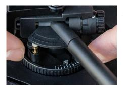
Set the anti-skating by turning the anti-skating adjustment ring (4) to the desired level. Anti-skating is generally set to the same level as your tracking force.
