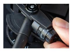
Once it is level, put it back in its rest. Turn the tracking force adjustment wheel (3) to set the desired tracking force.
