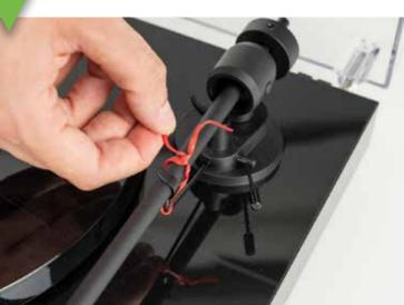
Remove the needle protection cover.
