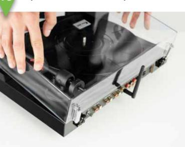
Plug in the power supply and connect the turntable with your speakers.
