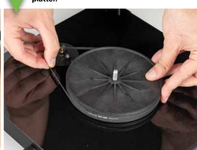
Put the platter on and remove tonearm protection.
