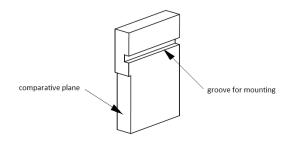
Step 1: Place the tool with groove to the headshell as shown.
