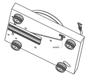
• Turn on the switch located in the bottom of plinth
