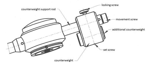
Put on counterweight on the support rod. Tighten the locking screw gradually and watch than the shaft entry into thread groove. Then tighten the locking screw. Correction of counterweight's weight is provided by additional counterweight is also tighten by the set screw.
