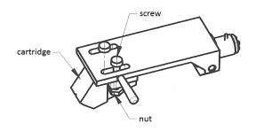
For cartridge assembly use fasteners from cartridge accessories. Fix the cartridge in the middle of headshell oval holes.
