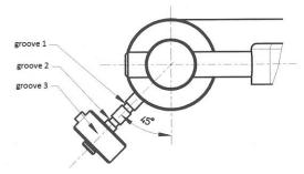
With the anti-skating slider adjust the position of the arm weight at 45 degrees.
