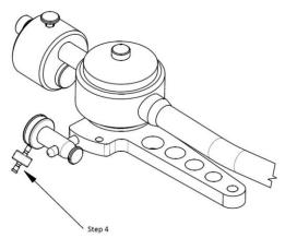
When the tonearm is over the first outer groove of the record, the anti-skating thread must be already tensioned, when it's in the end, it must be still on tension.
