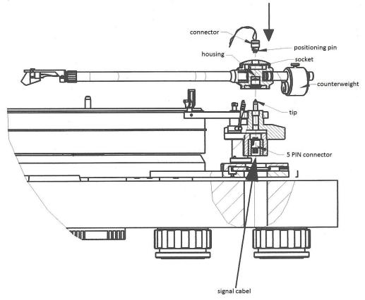
Insert output connector carefully into socket in housing. Positioning pin must be directed to cartridge counterweight. After insertion the connector into socket, lock the connector with fixing nut.
