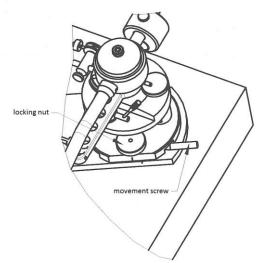
Loosen the locking nut allows the linear shifting of the tonearm. Adjust correct distance by using of the scale. The correct mounting distance 304.8 mm on the scale is valid only if the cartridge is in the correct position on the headshell.
