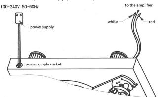
Turntable is supplied with a power supply suitable for your country's mains supply. Check the label before connecting to ensure compliance with the mains rating in your house.
