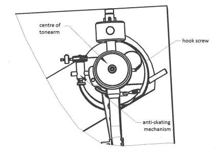
Assembly of anti-skating is described in the following four steps: **Step 1:** Mounting the thread on the hook screw
