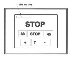
Touching on field 33 or 45 selects the desired speed. The display shows "WAIT". After reaching rated speed is displayed selected value 33,3 or 45,1. Rated speed can be correct by touching the + or -, which changes the value by 0.1 % Turn off or pause the recording, touch STOP.
