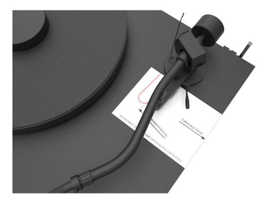
Loosen both VTA setting screws and carefully slide the arm toward the platter so that the tonearm support follows the new position shown on the template.
