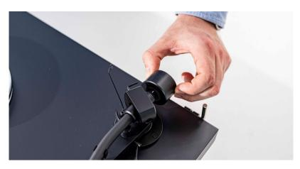
Pushing carefully, move the counterweight (6) onto the rear end of the counterweight support rod as shown in the picture below. Place the stylus pressure gauge onto the platter. To set the required VTF, lower the tonearm lift lever as indicated in the illustration and place the tip of the stylus exactly in the point marked 23mN (23mN = 2,3g). If the stylus gauge becomes level, then the correct pressure has been
