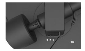
Slip the loop of the anti-skating weight's thread over the third groove of the stub to set the correct anti-skating force for the factory-fitted cartridge. Feed the thread through the loop of the wire support (17).
