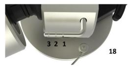
Slip the loop of the anti-skating weight's thread over the third groove of the stub to set the correct anti-skating force for the factory-fitted cartridge. Feed the thread through the loop of the wire support (17).
