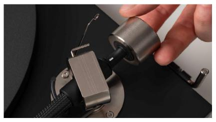
Pushing carefully, move the counterweight (6) onto the rear end of the counterweight support rod as shown in the picture below.
