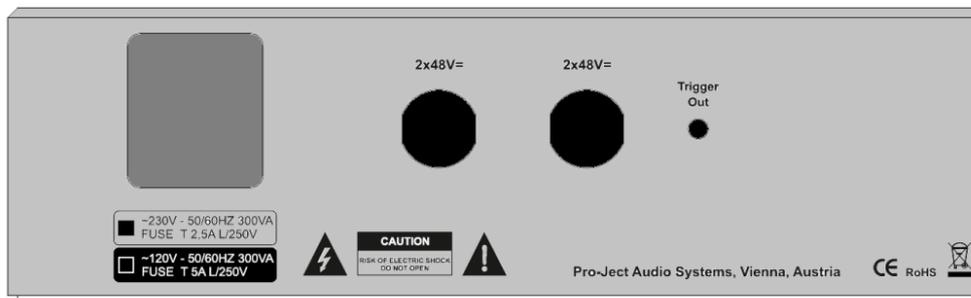
Pro-Ject Power Box DS2 Amp can power one stereo amplifier or two mono amplifiers.
