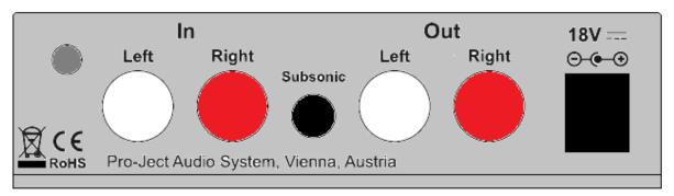
Make all connections whilst the phono amplifier is disconnected from the power supply. Take care to connect the left and right channels correctly. The right channel is usually marked red, the left channel black or white.
