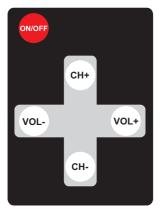
short press turns the unit on, long press takes it back into standby. Powered on, a short press activates and deactivates mute
