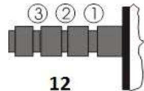
Slip the loop of the anti-skating weight's thread over the third groove of the stub to set the correct anti-skating force for the factory-fitted cartridge. Feed the thread through the loop of the wire support (14).
