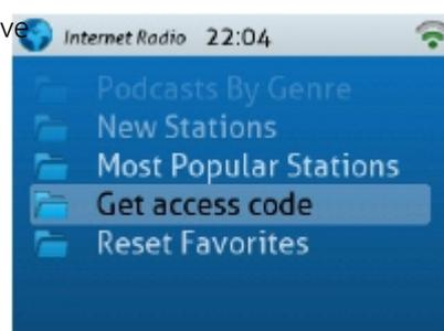
Now enter the access code you see in the Stream Box DS2 T display on the internet site <http://streamunlimited.vtuner.com>. DON'T use the code printed here in the manual, it will not work. On the vTuner website you have to register first (it's completely free of charge). Follow the instructions on the website for registering and compiling of the list.
