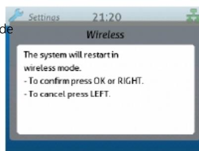
After the reset the Stream Box DS2 T shows the WLAN configuration menu. The symbol
