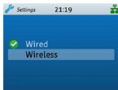
If the Stream Box DS2 T was in wired network mode before, the unit informs you, that it has to reset for a change to wireless connection mode. And asks, if you want it to do that. Please confirm with **OK**. The Stream Box DS2 T now performs a reset.
