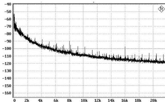
We can see that the noise floor at 1kHz is about  $-75\text{dB}$  and at 10kHz it is about  $-110\text{dB}$ .
