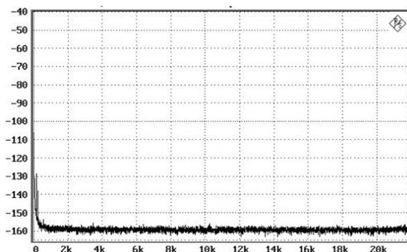
The results are limited by the capabilities of the measuring equipment and noise floor lays at  $-160\text{dB}$  or even lower. There are visible peaks at 50Hz and 100Hz which are caused by limits of the measuring instruments. However, they are at a level of  $-130\text{dB}$  and  $-140\text{dB}$ .
