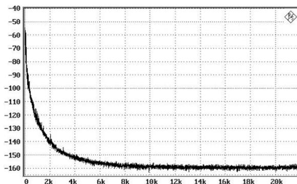
After applying passive RF interference filtering the results are already remarkable. Noise on 1kHz drops to  $-125\text{dB}$ , at 10kHz Noise comes even close to  $-160\text{dB}$ . But they improve even further when applying an active filter after the passive filtering.
