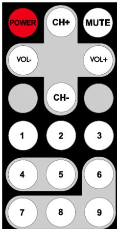
**POWER** turns the unit on or back into standby
