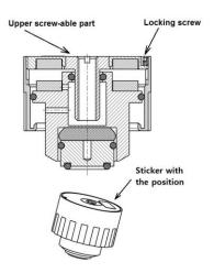
To adjust the feet, turn the small locking screw placed in the upper part of the feet about 180 degrees. Then screw the upper part by the screwdriver down to make the feet stronger.
