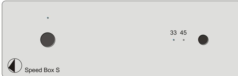
The belt must be on the smaller (50Hz models) larger (60Hz models) diameter part of the motor pulley. Press the button **33 45** to switch between 33 and 45 r.p.m.. The selected speed is shown respectively by the lit LED. To play at 45 or \*\* 78 r.p.m. please always start the turntable at 33 r.p.m. and then switch to the higher speed when it has attained full speed.
