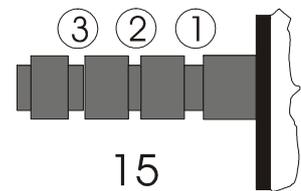
Hang the loop of the thread of the anti-skating weight into the groove of the anti-skating stub (15) corresponding to the downforce applied to your cartridge and hang the thread in the groove of the wire support (17).
