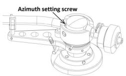
With the aid of a good magnifying glass adjust the needle until it is vertical in the groove (i.e. perpendicular to the record's surface). Ideally this should correspond to the top surface of the cartridge body being parallel to the record surface.
