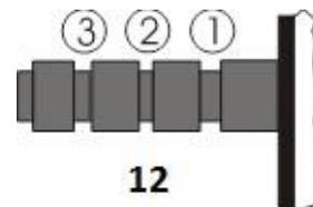
Hang the loop of the thread of the anti-skating weight into the groove of the anti-skating stub (12) corresponding to the downforce applied to your cartridge and hang the thread in the groove of the wire support (14).
