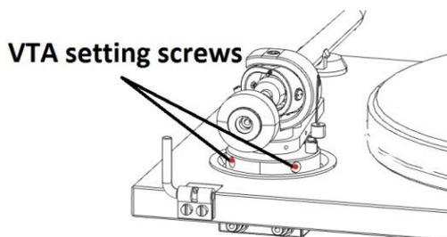
Retighten the hexagon screws without applying excessive force (which would deform the arm pillar) – finger tight is quite sufficient.
