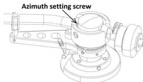
With the aid of a good magnifying glass adjust the needle until it is vertical in the groove (i.e. perpendicular to the record's surface). Ideally this should correspond to the top surface of the cartridge body being parallel to the record surface.
