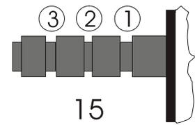
Hang the loop of the thread of the anti-skating weight in the groove of the anti-skating stub (15) corresponding to the downforce applied to your cartridge and feed the thread through the loop of the wire support (17).
