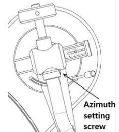
With the aid of a good magnifying glass adjust the needle until it is vertical in the groove (i.e. perpendicular to the record's surface). Ideally this should correspond to the top surface of the cartridge body being parallel to the record surface.
