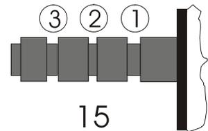
Slip the loop of the anti-skating weight's thread over the second groove of the stub to set the correct anti-skating force for the factory-fitted cartridge. Feed the thread through the loop of the wire support (17).
